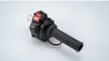
APS "Accelerator Position Sensor"
